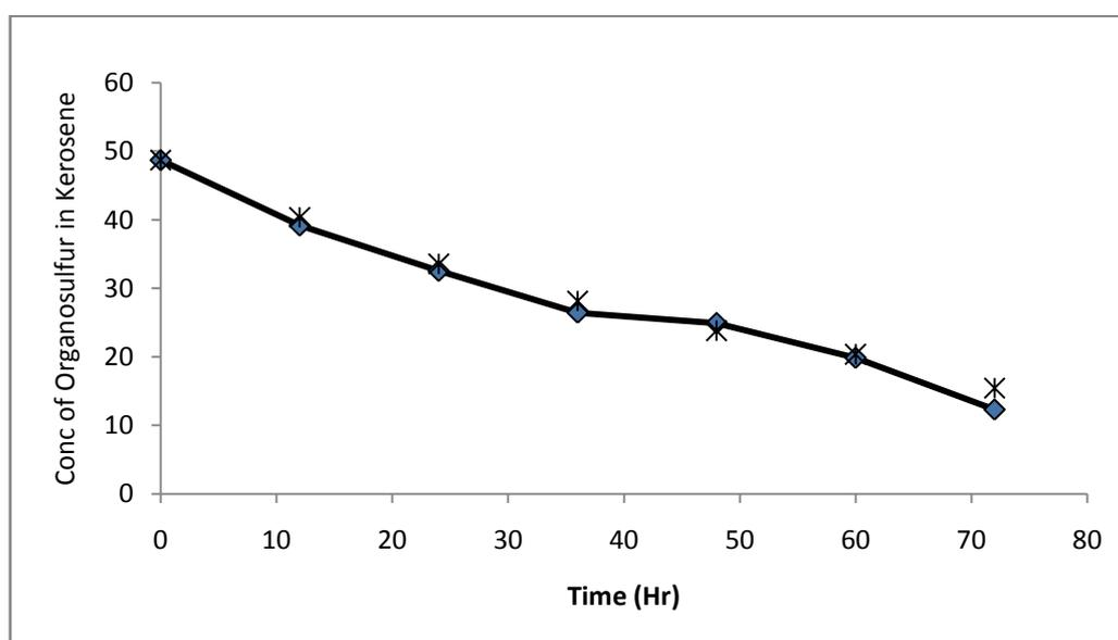
Figure 1: The Experimental and Simulated Concentration – Time Profile Kerosene Bio desulfurization by *D indolicum*.
